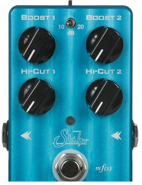
**On/Off Effects Status Indicator:** The LED indicator displays Dual Boost's effect status, on/off, as well as the current channel [Green (Boost 1) or Red (Boost 2)].
