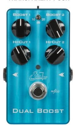
When set to the more mild 10dB boost range, the Dual Boost compliments the interaction between your guitar and amplifier, enhancing playability while retaining dynamics.
