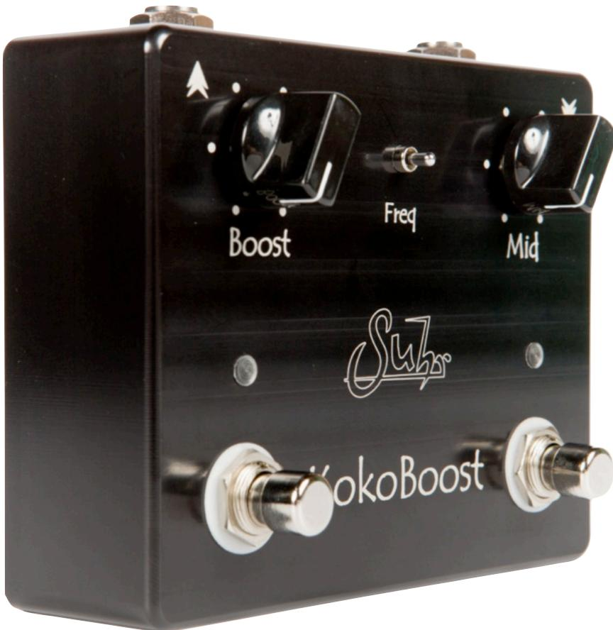
**True Bypass:** True bypass can be defeated, allowing the pedal to be used as a buffer by switching the internal True Bypass/Buffer switch. Remove the cover and set the switch located between the 1/4" jacks.
