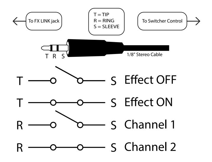
A connection between the Tip and Sleeve controls Alexa's ON/OFF state.
